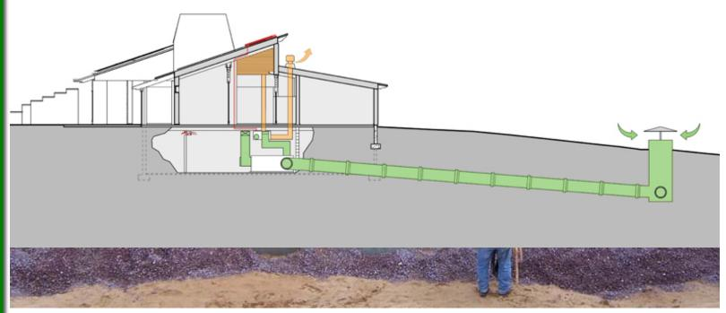
Installation of large earth ducts to preheat and precool the air.
