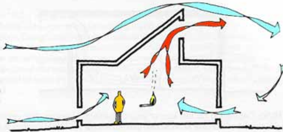
Figure 15.27: A high window acting as a windscoop inlet together with a low outlet must overcome the stack-effect tendency of the warm inside air to rise; reorienting the windscoop to leeward reinforces the stack effect and increases airflow.
