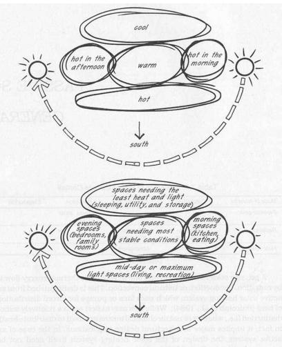
Figure 7.2: Designing for the sun: (a) horizontal temperature zones of building interiors, and (b) potential design response. (After AIA, 1981.)
