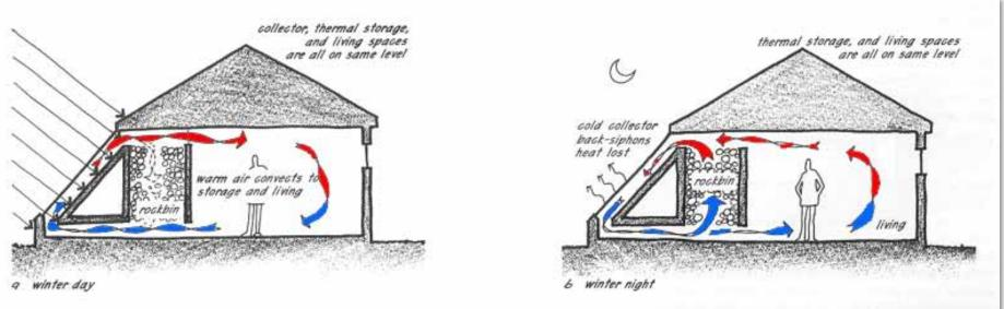
Figure 11.1: Positioning the collector, storage, and living areas at the same level in a convective air loop system: (a) winter day operation — level arrangement allows convective heating to occur during the day; (b) winter night operation — this "level" positioning of components permits unwanted back-siphoning, effectively cooling the system.
