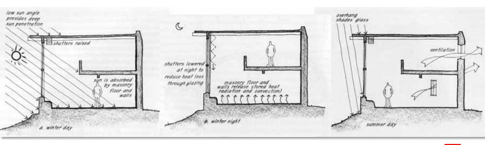
The direct gain system makes overt use of solar geometry to ensure that sun reaches the thermal mass in the winter, and that shading devices prevent solar access during the months where cooling is the dominant issue.
