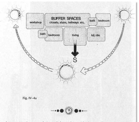
Locate openings to admit sunlight and provide for ventilation—WINDOW LOCATION(6)—while at the same time choosing the most appropriate heating system for each space—CHOOSING THE SYSTEM(7). If a greenhouse is integrated into the building—SIZING THE GREENHOUSE(15)—place it along the south face of the building for maximum exposure to the winter sun.
