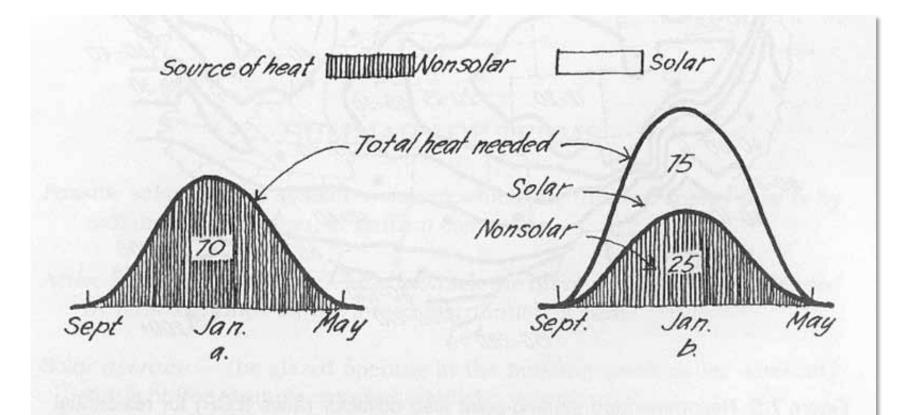
Figure 7.4: Performance comparison of: (a) "reference" non-solar building and (b) passive solar building. (Redrawn from Stein et al., 1986, by permission.)
