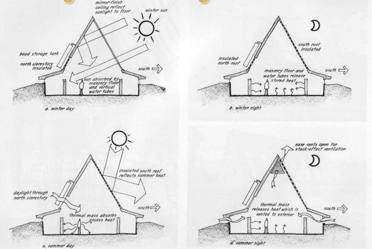
Figure 8.8: Patoka Nature Center modes of operation: (a) winter day, (b) winter night, (c) summer day, and (d) summer night. The building uses "night flushing" as a summer ventilation cooling strategy. Sixteen small awning windows over the exhibit booths admit air while large louvered exhaust eave vents are very effective in inducing stack effect night ventilation during the summer.
