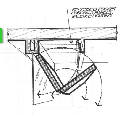
FIG. 39c. Hinged and fold-down panels offer large additional resistances to window units, can be made from aluminum-faced urethane or polystyrene sandwich panels, or insulation board w/laminated facings.
