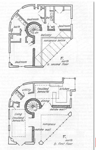
Figure 10.4: "Unit One" — First Village (a) upper, and (b) lower floor plans. (Redrawn from Howard and Fraker, 1990, by permission.)
