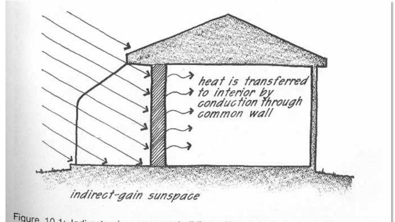
Figure 10.1: Indirect-gain sunspace building with common thermal storage wall. Conduction through the common wall is the primary means of heat transfer to living space.
