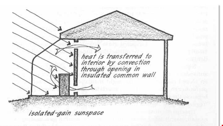
Figure 10.2: Isolated-gain sunspace building with free-standing thermal storage mass and insulated common wall. Convection (either fan-forced or natural) is the primary means of heat transfer to living space.
