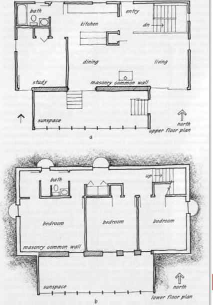
Figure 10.8: Solargreen floor plans: (a) upper level, and (b) lower level.
